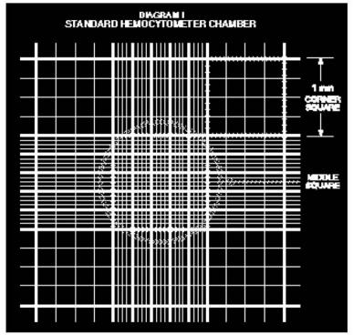
The circle indicates the approximate area covered at  $100 \times$  microscope magnification ( $10 \times$  ocular and  $10 \times$  objective). Include cells on top and left touching middle line ( $\bigcirc$ ). Do not count cells touching middle line at bottom and right ( $\bigcirc$ ). Count 4 corner squares and middle square in both chambers (one chamber represented here).
