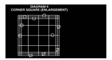
Count cells on top and left touching middle line ( $\bigcirc$ ). Do not count cells touching middle line at bottom and right ( $\varnothing$ ).
